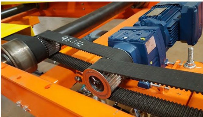
▲ Close up of a Power Roll Bed drive frame showing a gearmotor, double pulley and drive belts.
