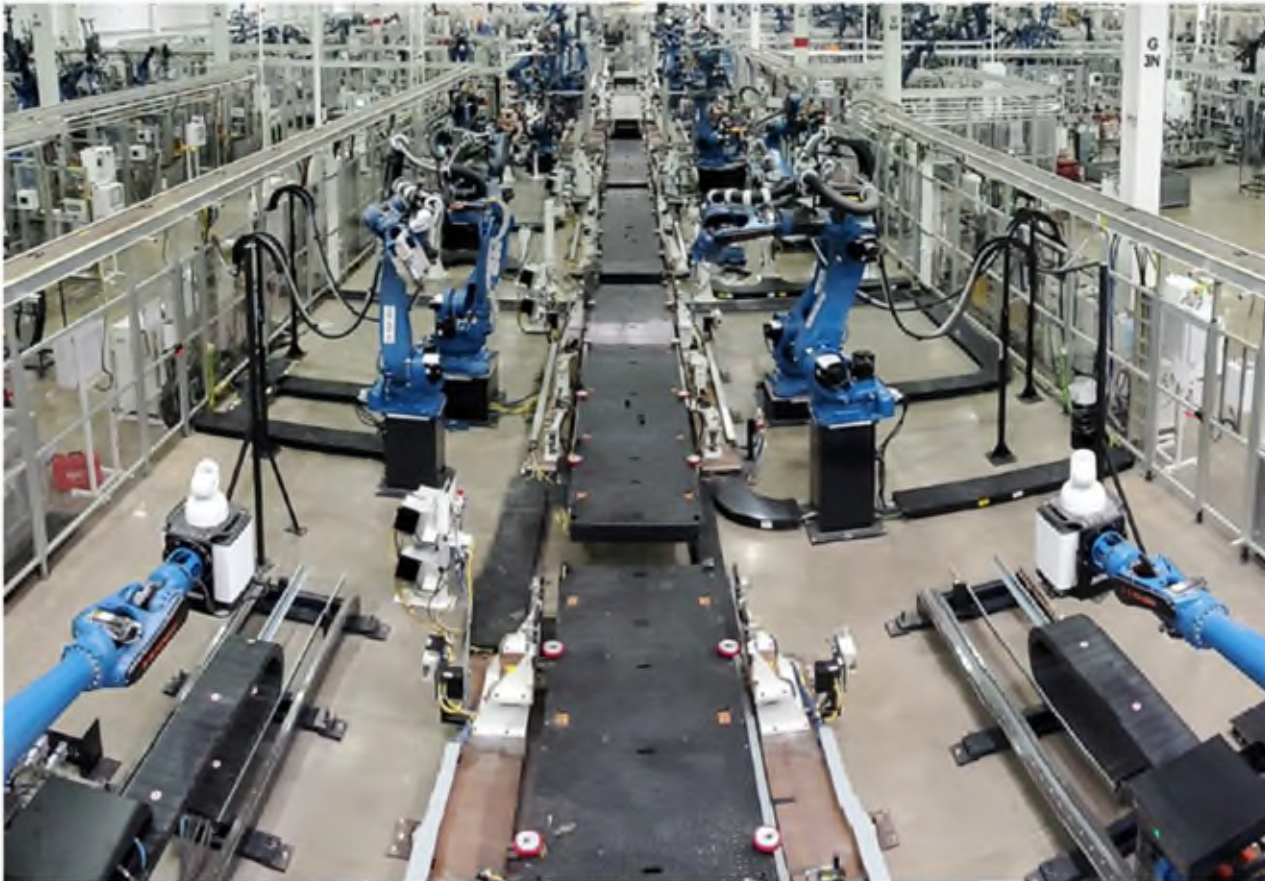
▲ Power Roll Beds as shown with robots in an automotive body shop.
