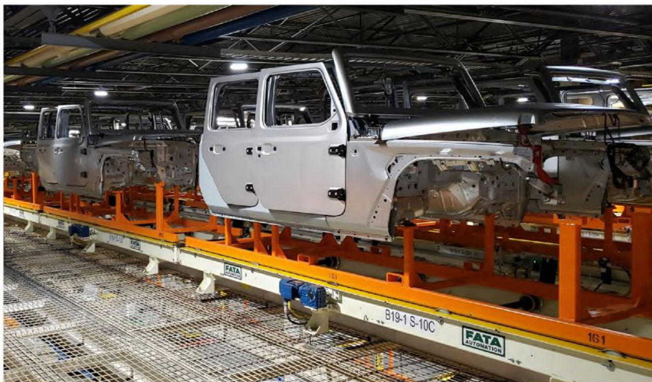
▲ Power Roll Beds shown carrying vehicle bodies in an automotive plant.
