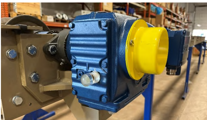
▲ Power Roll Bed with drive mounted externally.
