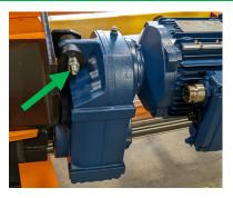
Insert and tighten the screw to 88 Nm that connects the gearmotor to the drive shaft.
