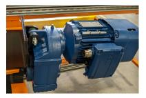
7 Install the new gearmotor onto the drive shaft, after checking parallel key for integrity.
