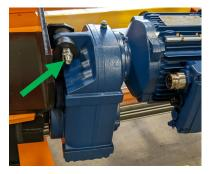
Remove the gearmotor from drive shaft.
