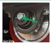
Pull the drive shaft through the pillow block bearings and drive wheel until you are able to lower the drive wheel out of the drive wheel block.
