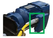
3 Remove the drive shaft cover on the gearmotor.
