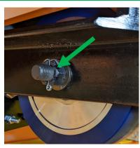
Install and secure the idle wheel block onto the trolley with the four screws and washers from step 0. Apply removable Loctite onto the screws before inserting and tighten these screws to 330 Nm.
