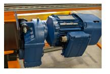
Loosen and remove the four screws holding the drive wheel block to the trolley, and transfer the drive wheel block to a workbench.
