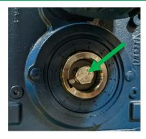
5 Loosen the nut and bolt that holds the gearmotor to the trolley.
