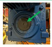
6 Loosen and remove the screw that connects the gearmotor to the drive shaft.
