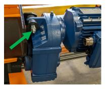
Remove the gearmotor from drive shaft.
