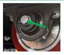
Install and secure the drive wheel block onto the pivot table with the four screws and washers from step 9. Apply removable Loctite onto the screws before inserting and tighten these screws to 330 Nm.
