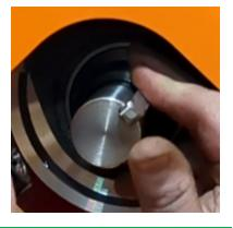
Insert and tighten the nut and bolt that holds the gearmotor to the trolley.
