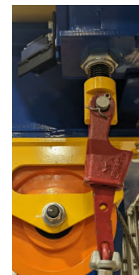
Fixing pin attached to a tension/slack switch
