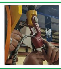
After the rope is secure there may be a small gap at the top. This can be corrected by applying the load of the carriage, afterward the rope will be properly seated within the attachment point.
