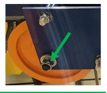
Remove the M16 bolts (5) fixing the pulley assembly to the 4-Post Lift frame.
