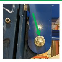
Remove any gearmotor supports from the service rail.
