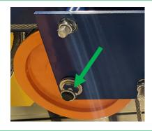
Remove the M16 bolts (5) fixing the pulley assembly to the 5 4-Post Lift frame.
