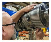
When wrapping the ropes, the outer wraps should extend from the top of the drum out towards the wide pulleys and the inner wraps should extend from the bottom of the drum out towards the narrow pulleys.
