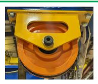
Torque the M16 bolts (4) to 219 Nm and secure the frame drop pulley to the frame.
