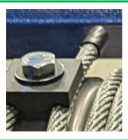
Run the motor and drive the drum to wrap the rope. Hold the rope under tension while the rope is wrapped.
