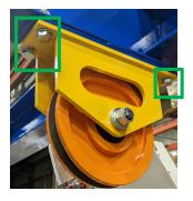
Torque the M20 bolt to 441 Nm and secure the pulley wheels with the wire ropes.
