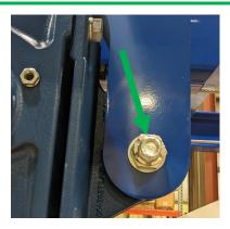
4 Remove the M16 bolts (4) to free the motor from the plate.
