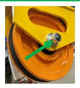
Remove the M16 bolts (4) fixing the pulley assembly to the 4-Post Lift frame.
