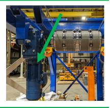
Place the cap and torque the M16 bolt to 219 Nm to attach the motor to the shaft.
