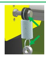
2 Remove and replace the tension spring.
