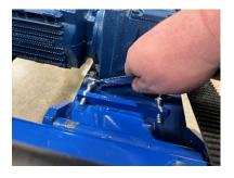
9 Place cover back on power roll bed and tighten screws.
