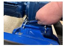
4 Hoist gearmotor and remove belts from pulley.
