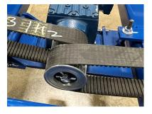
Hand-tighten the four gearmotor mounting bolts and adjust alignment with horizontal hex-head screws. Adjust drive pulley to roller pulleys, so they are straight and square for proper operation. Then tighten the four mounting bolts completely.
