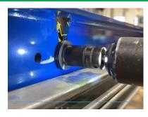
5 Lift roller shaft upward and remove one end of the belt. Perform the same to belt sharing roller shaft.
