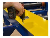
Both belt sharing rollers of the damaged belt will need to beloosened from the frame to free up any tension and to replace the belt.
