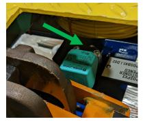
Remove the M10 bolts (4) from the clamp mounting bracket and then remove the clamp.
