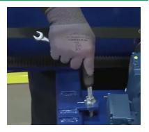
If a belt cannot become correctly tightened (<10Hz), then the belt is to be replaced.
