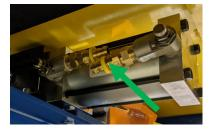
3 Disconnect the cords from the cylinder position sensors.
