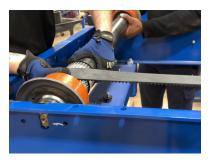
Remove damaged belt and replace with new one. Thread each roller through the toothed belt(s) so that they are on the appropriate pulleys and rollers.
