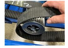
Remove head screw and split pin to dismantle pulley from old gearmotor. Install pulley with a new split pin on new gearmotor.
