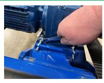
Once the large belt tension is sufficient, adjust the tensioner to achieve the desired tension for the small belt.
