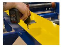
Loosen screws at one side of the motor. Then proceed to remove mounting bolts.
