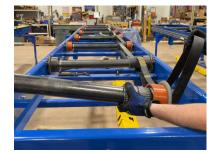
Insert new roller through the toothed belt(s) and place it on the pulley.
