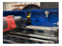
8 Place cover back on power roll bed and tighten screws.
