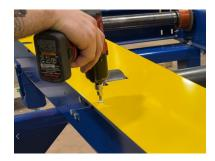
Remove the hex head screws holding the shafts on both sides of the roller. To replace an interior roller, the belt sharing rollers may also need to be loosened from the frame to free up tension from the belts.
