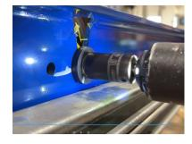
4 Lift roller shaft upward and remove belt(s) off roller shaft.
