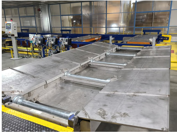
▲ Power Roll Bed Wet Application showing stainless steel rollers and optional stainless-steel wings.
