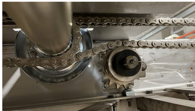
▲ Close-up of stainless-steel roller and chain tensioner on Power Roll Bed WA.
