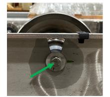
Remove the M10 screws holding the flanges on both sides of the worn roller.
