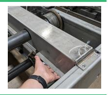
Place any covers back on the Power Roll Bed and tighten screws.
