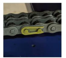
4 Open the master link of the chain on both sides of the roller.
