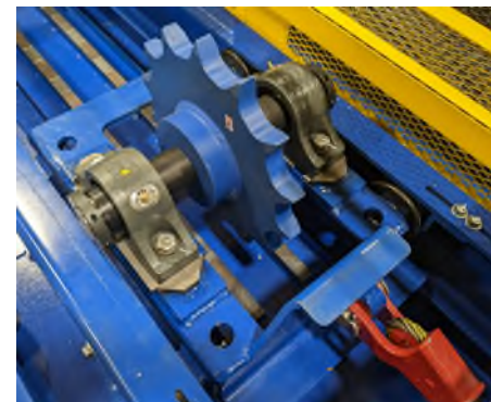
▲ Take-up float frame assembly
