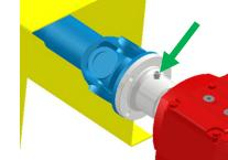
Undo the setscrew in the cardan shaft and remove the universal 4 joints from gearmotor shaft.
