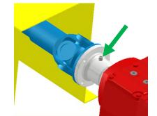
**9** Tighten the set screws on the cardan shaft flange.
