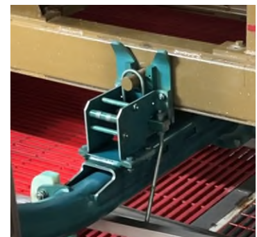
Skid-Locking Mechanism with a skid
