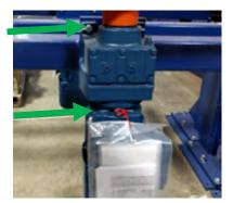
4 Support the gearmotor then remove the bolts (4) in the gearmotor.
