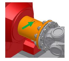
**11** Tighten the set screw for the companion flange.
