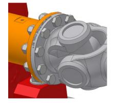
6 Return and tighten the M16 bolts (10) securing the cardan shaft to the companion flanges on both ends.
