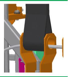
25 Wrap one end of a belt around the turnbuckle
