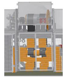
**32** Install the counterweight safety panel and the polycarbonate panel assembly that were removed earlier.
