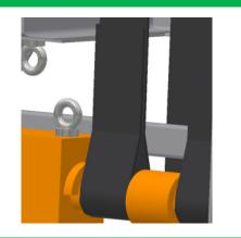
**15** Wrap one end of a belt around the top of the counterweight.
