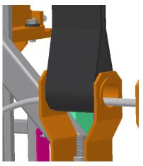
Place the clamping plates with the bottom of the clamp plates four 26 (4) inches above the top of the turnbuckle.
