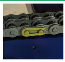
5 Reinstall the new chain with the master link.
