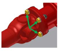
6 Loosen and remove the M8 mounting bolts (4) securing the motor to the pedestal.
