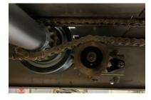
In order to replace a roller, all adjacent rollers must be disassembled that are mounted at the respective gearmotor side.
