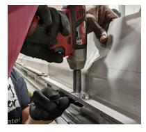
3 Adjust the tensioner to loosen the chain.
