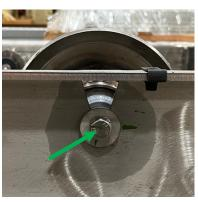
Turn around flanged bearings 90°, to get them through the cutout of side frames. If they are clamped between side frames, you must loosen screws of drive shaft and pull bearings slightly apart, so that the carrying roller can be withdrawn upwards.
