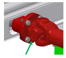
4 Loosen and remove the M8 bolts (8) attaching the cardan shaft to the companion flanges at both ends.
