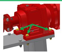
7 Remove the original gearmotor and replace with the new one.
