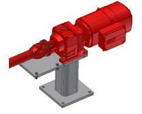
8 Set and tighten the M8 mounting bolts (4) to 25Nm securing the motor to the pedestal.
