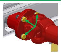
7 Tighten the setscrews in the flange at both ends of the cardan shaft.
