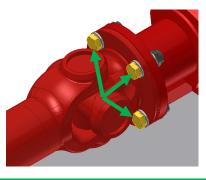
Tighten the setscrews in the flange at the gearmotor end of the cardan shaft.
