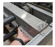
3 Remove the tensioner to relieve tension on the chain.
