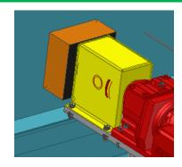
**12** Remove the gearmotor support.
