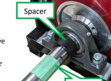
Pull the drive shaft through the pillow block bearings and drive wheel until you are able to lower the drive wheel out of the drive wheel block.
