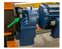
5 Loosen the nut and bolt that holds the gearmotor to the trolley.
