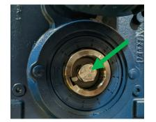
Insert and tighten the screw to 88 Nm that connects the 17 gearmotor to the drive shaft.
