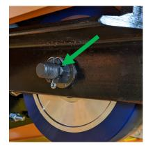
Remove the cotter pin holding the slotted nut in place.Loosen and remove the nut.
