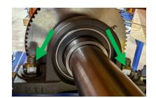
**11** Tighten all the M20 bolts for the pillow block bearings.
