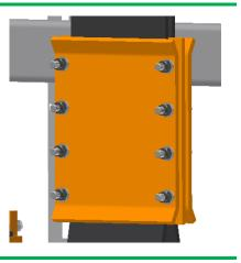
Place the clamping plates with the bottom of the clamp plates four(4) inches above the top of the turnbuckle.
