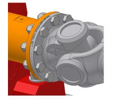
Return and tighten the M16 bolts (10) securing the cardan shaft to the companion flanges on both ends.
