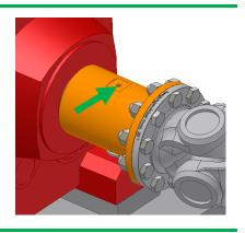
Pull the cardan shafts away from the gearmotor to free the companion flange from the gearmotor shaft.
