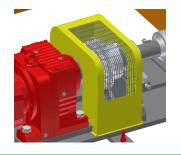
**11** Return the standby drive chain coupling guard to the closed position and secure it.
