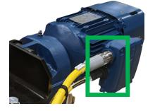
3 Loosen the M10 bolts in the motor mount and remove the bracket below.
