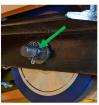
Remove the M25 shoulder screw that serves as the axle for the idle wheel.
