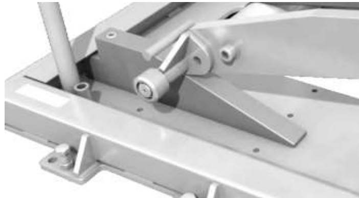
Fig. 23: For maintenance purposes, maintenance wedges relieve the load on the rollers and rails
