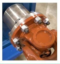
Replace and tighten the M8 bolts securing the guard over the cardan shaft.
