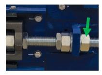
Tighten the inside nut evenly on both sides of the Cross-Conveyor Take-Up until the belt is at the required tension.
