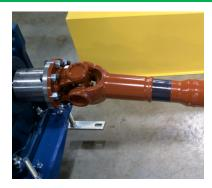
Remove the M24 bolts (4) securing the gearmotor to the base plate.
