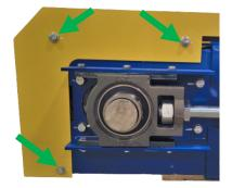
Undo the hexagonal head nuts on the tension unit to slacken the Chain.
