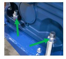
**7** Replace the original gearmotor with the new one.
