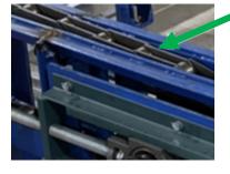
5 Replace the Chain and check the number of chain link before installation it.
