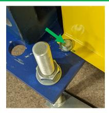
4 Loosen the lock nuts and set screws from the companion flanges at the gearmotor ends for both cardan shafts.
