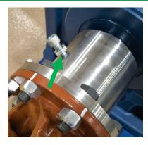
Torque the M24 bolts (4) securing the gearmotor to the base plate.
