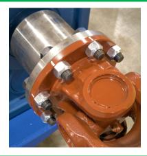
4 Remove and replace the cardan shaft.
