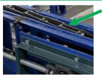
7 Tighten the hexagonal head nuts to tension the Uni-Chain until the chain can be deflected by the thickness of a finger.
