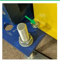
Remove the bolts securing the cardan shaft to the companion flanges on both ends.
