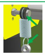
2 Remove and replace the tension spring.
