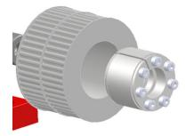
Align the drive pulley so that the lifting belts will run in the center.
