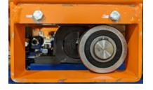
5 Remove the belts off the drive pulley.
