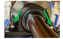
Pull the lifting cam assemblies slightly to the center of the lift to reduce tension on the lifting belts.
