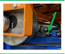
4 Loosen the pillow block bearing M16 bolts for all the pillow block bearings.
