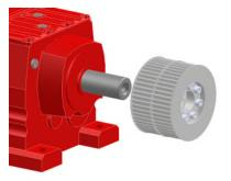
8 Remove the clamping set and inspect for damage. Replace if necessary.
