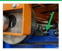
3 Loosen the pillow block bearing M16 bolts for all the pillow block bearings.
