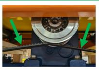
7 Inspect the lift pulley, cam rollers, and the drive pulley for wear and damage. Replace as necessary.
