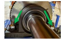
Pull the lifting cam assemblies slightly to the center of the lift to reduce tension on the lifting belts.
