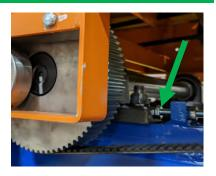
Loosen the pillow block bearing M16 bolts for all the pillow block bearings.
