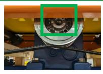
7 Pull the original drive pulley off the motor drive shaft.
