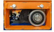
Tighten the inner jack screws evenly keeping the lift pulleys parallel with the drive pulley until the lift belts are properly tensioned. If necessary, adjust the outer jack screws.
