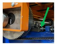
14 Tighten all the M20 bolts for the pillow block bearings.
