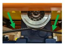
Loosen and remove the M16 bolts (4) that hold the lift motor to the lift table base.
