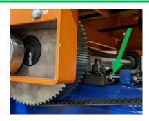
13 Tighten all the M20 bolts for the pillow block bearings.
