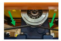
Tighten the inner jack screws evenly keeping the lift pulleys parallel with the drive pulley until the lift belts are properly tensioned. If necessary, adjust the outer jack screws.
