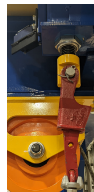
▲ Fixing pin attached to a tension/slack switch
