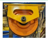
Torque the M16 bolts (4) to 219 Nm and secure the frame drop pulley to the frame. **17**
