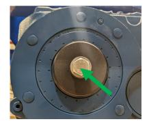
Place and torque the M16 bolts (4) to 219 Nm to attach the motor to the plate.
