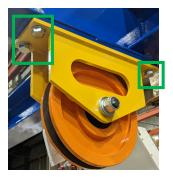
Torque the M20 bolt to 441 Nm and secure the pulley 18 wheels with the wire ropes.
