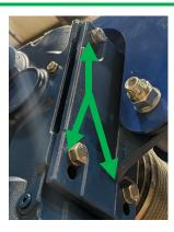
Place and torque the M24 bolt to 762 Nm to attach the motor to the motor mount.
