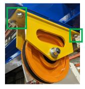
Remove and replace the frame drop pulley assembly.
