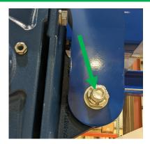
6 Remove the M16 bolts (4) to free the motor from the plate.
