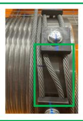
After completing the second wrap through the wire clips, torque bolts down (55 Nm) with tension on the rope.
