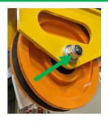
Remove the M16 bolts (4) fixing the pulley assembly to the **15** 4-Post Lift frame.
