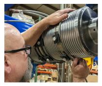
When wrapping the ropes, the outer wraps should extend from the top of the drum out towards the wide pulleys and the inner wraps should extend from the bottom of the drum out towards the narrow pulleys.
