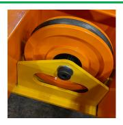
Torque the M16 bolts (5) to 219 Nm and secure the carriage drop pulley to the frame.
