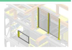
Remove any gearmotor supports from the service rail.
