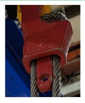
Wrap the excess rope. Cut and cap only after ensuring carriage is level in next steps.
