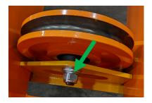
Remove the M16 bolts (4) fixing the pulley assembly to the carriage frame.
