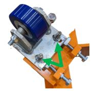
**3** Remove the original assembly and replace with a new one.
