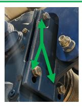
Remove the M16 bolt and cap to free the motor from the shaft.
