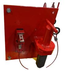
Remove the safety pin from its stowed position on the lock pin bracket and completely insert it into the locking position. The end of the safety pin should protrude though the locking slot.
