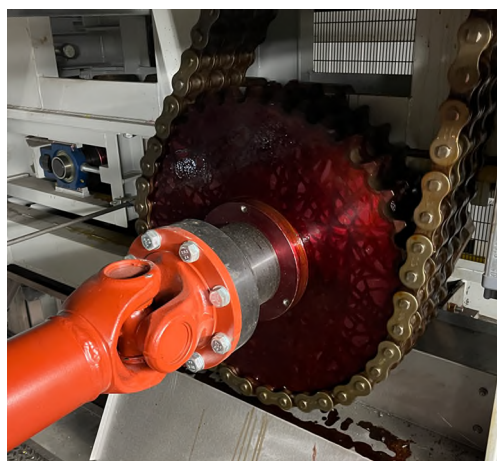
▲ Lower Caterpillar Drive Assembly – Cardan Shaft and Drive Sprocket
