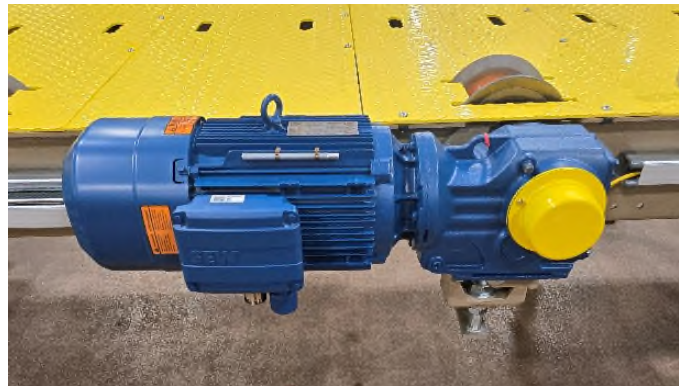
▲ Power Roll Bed with drive mounted externally.
