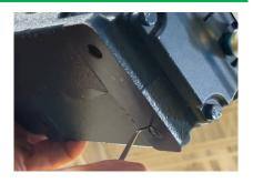
Apply Loctite to the bolts intended for securing the gearmotor base to the bottom of the gearmotor.
