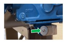
Remove the retaining pin from the frame and the gearmotor base.
