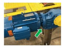
4 Remove all screws to remove the gearmotor cover.
