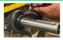
Remove the protective shipping caps and 15 the contents of the hollow bore in the SEW gearmotor.
