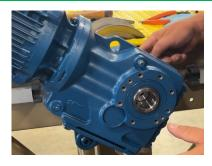
Align the mounting holes on the newgearmotor base with the holes on the conveyor frame.
