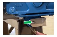
8 Using an overhead crane, carefully hoist the gearmotor off the unit.
