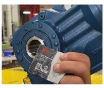
Remove the retaining ring from the hollow bore and set it aside.
