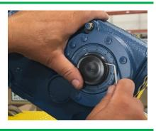
Set aside the SEW provided NOCO-Paste corrosion protection and lubricant.
