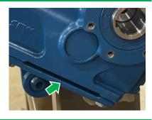
Using a fine-grit sand disk, gently cleanthe external drive shaft to remove any material buildup.
