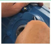
Remove the screw plugs from the bottom of the gearmotor as well.
