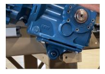
Reinsert the retaining pin on the frame and the gearmotor base.
