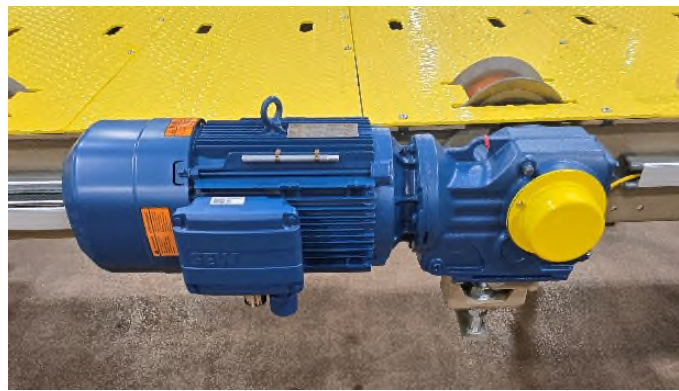
▲ Power Roll Bed with drive mounted externally.
