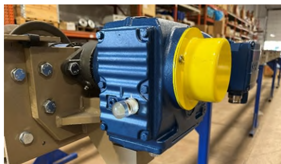
▲ Power Roll Bed with drive mounted externally.
