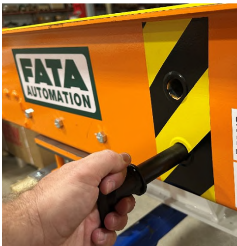
◀ A Safety Pin with slots directly on the frame
