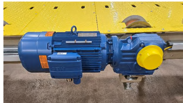
▲ Power Roll Bed with drive mounted externally.
