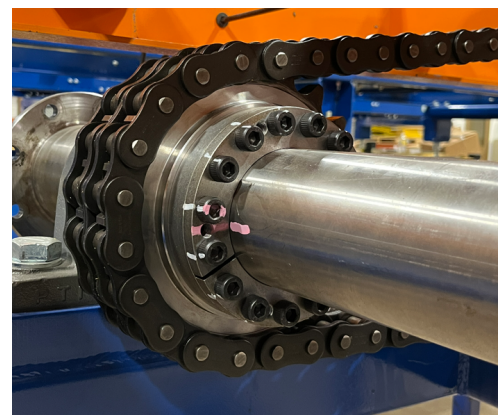
Close up of the drive sprocket.
