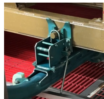
▲ Skid-Locking Mechanism in Locked position.
