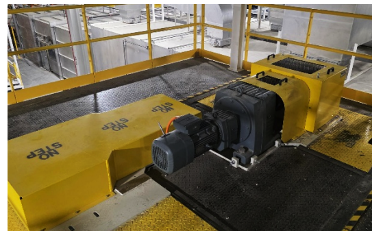
▲ Drive Assembly for PTED System at Scout
