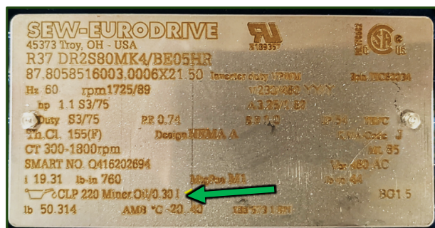
▲ SEW Gearmotor Data Plate Example
