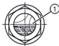
Figure 10-6 Oil level in the oil sight glass
