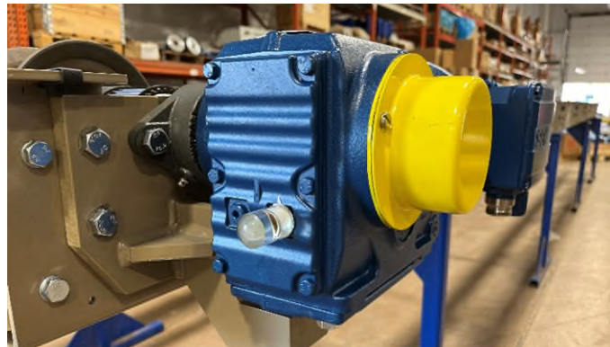
▲ Power Roll Bed with drive mounted externally.
