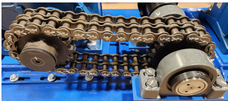
▲ Drive Sprocket and Guide Roller
